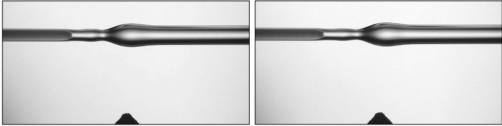
Fig. 30. Splice after additional heating No. 2 (left) and No. 3 (right).
