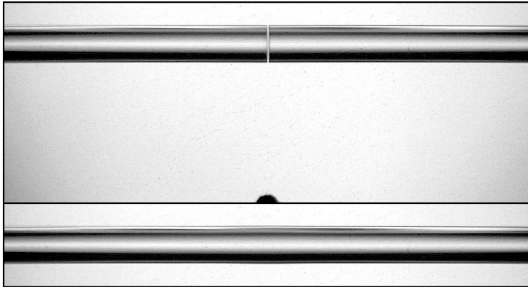
Fig. 1. Two identical 125 \mu\text{m} silica fibres before (top) and after (bottom) arc fusion. Electrode tip is visible as a black spot at the bottom of upper image.
