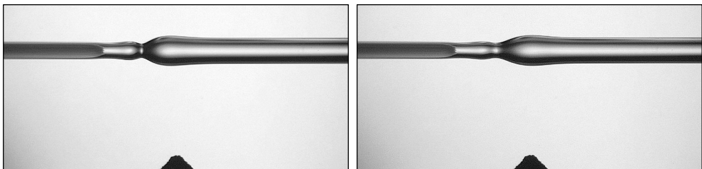
Fig. 29. Left: fibres fused. Right: splice after additional heating No. 1.
